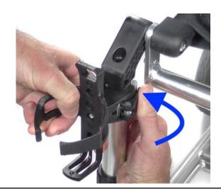
If the clamp is not tight enough, open the lever and rotate it one more turn to the right.
