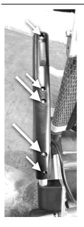
**3.** Remove the screw **D** to separate the control handle from the metal lever arm.
