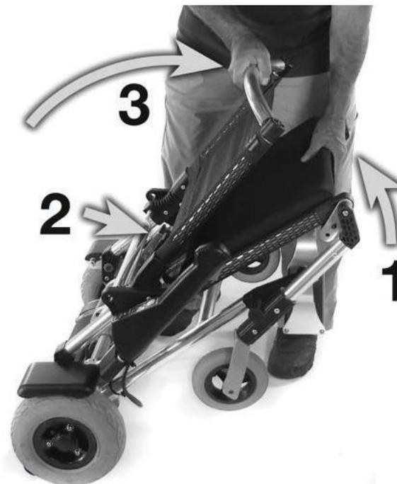
**NOTE:** *The parking brakes should automatically set each time the Zinger is unfolded, but always double check before sitting.*
