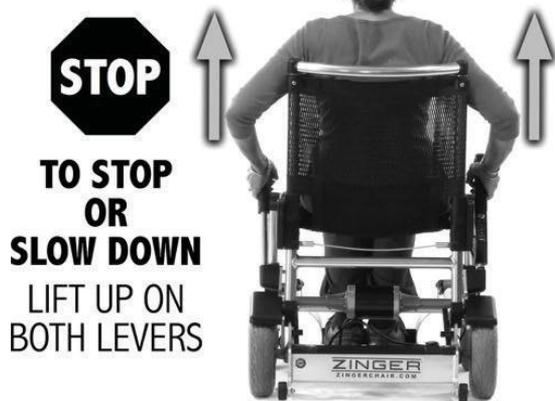
**NOTE:** Remember that the brakes will always apply when both levers are pulled back. If you have any confusion, just pull up on **BOTH** levers to brake!
