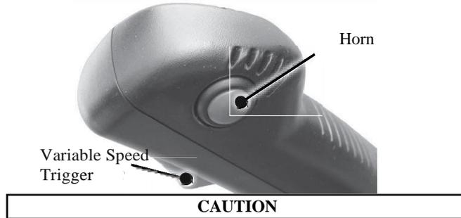
*Use minimal force when pressing the control buttons. Use the pad of your finger instead of a fingernail. Needless pressure or use of fingernails can lead to excessive wear and failure of the control buttons. After pressing a button, wait three seconds for the Zinger to respond.*
